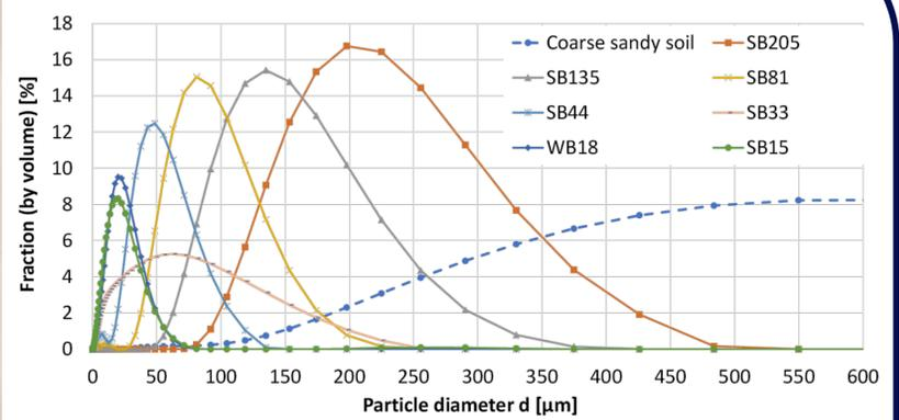
Particle size distribution curves of the different biochars used in the experiments and of the coarse sandy soil
