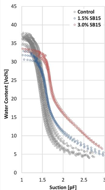
Soil water retention as a function of suction, with different dosages of the smallest straw biochar particles (15 µm median particle size)
