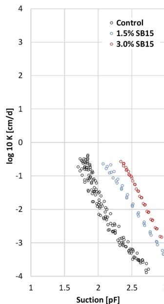
Unsaturated hydraulic conductivity as a function of suction
