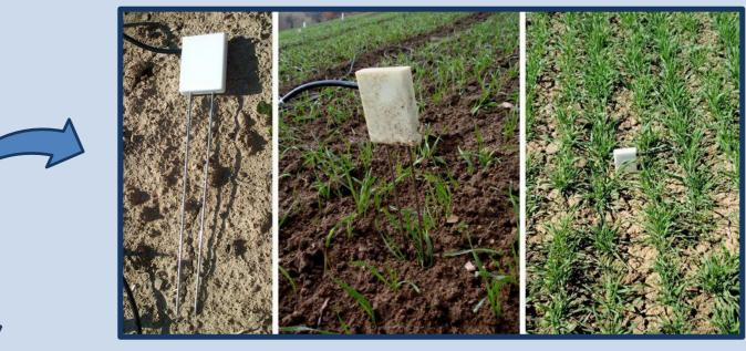
In each variant were sensors TDR to measure the soil water content placed vertically to monitor the soil water content from the surface to a depth of 30 cm.
