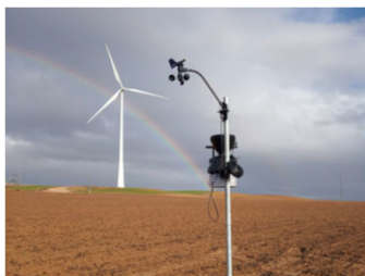
In November 2019, Bhupjit from Technical University of Denmark (DTU) was visiting one of the demonstration fields in Spain close to Madrid for installing soil sensors, a weather station, and a LoRaWAN gateway implementing wireless infrastructure. The farmer took part in the work.
